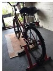
My go to for efficient exercise now.... Old bike sitting idle in the shed, triangle frame lifting the back wheel off the ground.
